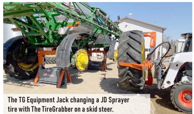
The TG Equipment Jack is designed specifically for the large Sprayers.
