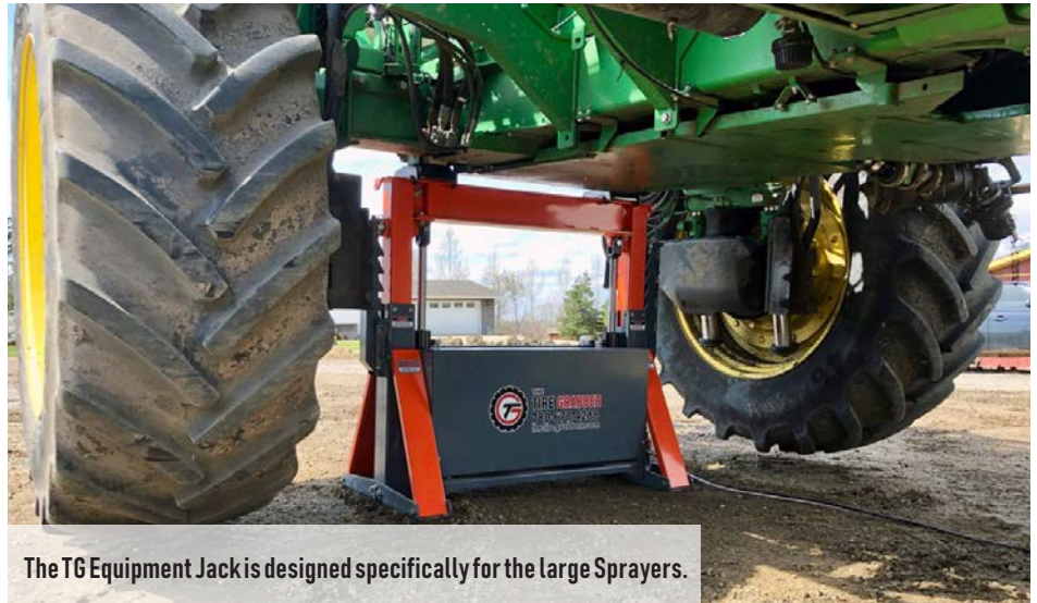
JD Sprayer changeover and the proper way to stack tires on a skid.
