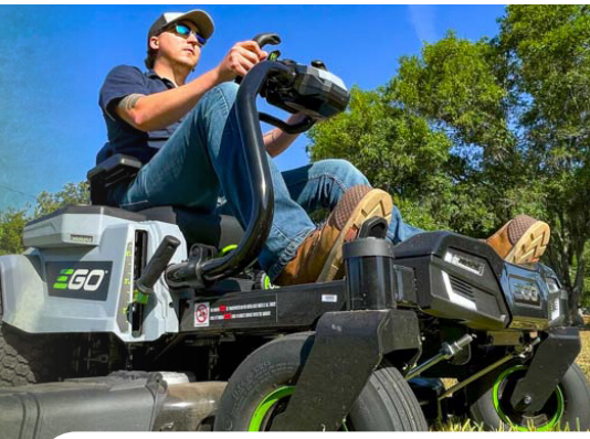
Shown above, the EGO POWER+ 42" Z6 ZERO TURN MOWER. For example, one of the six batteries used to power it is 56 volts. Because OSHA defines a high-voltage battery as 50v or more, this puts each of those six batteries in that category.
